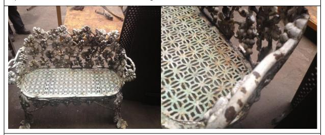
The course of treatment that we recommended to the customer was to blast off the existing coating(s) and take the bench back to bare metal. This required some delicate manual blasting by our blasters due to the age of the bench and the delicacy of some of the fine casting.
