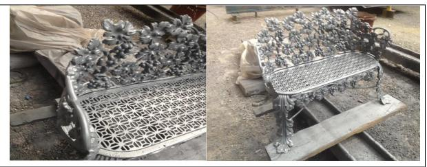
Once blasted and primed it became clear that there were areas of blow holes in cast iron work, this is when holes and blemishes open up in the metal. This can lead to future areas of paint breakdown and also affect the aesthetics of the finished job. Once the primer had cured the painter set about filling the blow holes with epxoy filler.
